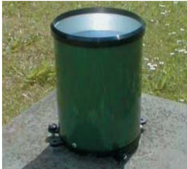
Advanced tipping bucket rain gauge
