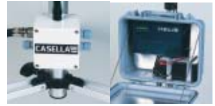
Sensor extension unit Sensus logger enclosure
